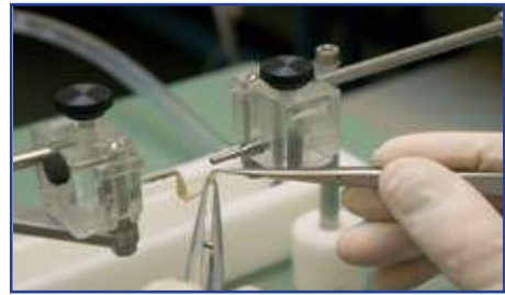
Figure 4.2. The blood vessel is connected to the tubes. Using 3/0 Prolene sutures the blood vessel is tightly fixated to the hollow tubes.
