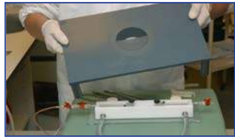
Figure 4.3. The tubes are gently laid within the blood vessel holder. to enhance the difficulty level, a trestle with a hole can be placed over the setup. The height of the trestle is adjustable (6-10 cm above the blood vessel).
