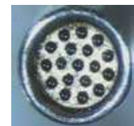
Grid H (similar to grid B, however, twice as thin) Surface. = 0.565 mm 2 .
